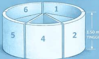
6 Molds = 1 Complete Tank 6 CETAKAN = 1 TANGKI LENGKAP
